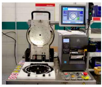
Each distributor is individually tested by a special machine to make sure that all parameters are respected (vacuum operation, tollerances, torque etc). If the test is succesfully passed, a sticker will be put on the distributor to certify quality control.
