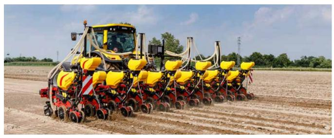
The beating heart of every precision planter is the distributor. MaterMacc was the first company to use high quality nylon polymers with fibreglass for the main components. This design guarantees long life operation and resistance to deformation, tear and wear. The company's belief is that, besides being at the cutting
